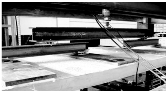
Figure (2). Test Setup Showing Loading Frame.
